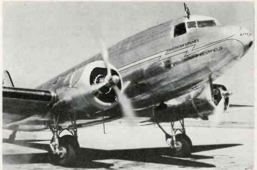
Airliner showing main transmitting and receiving antenna and two "Belly T" antennas
