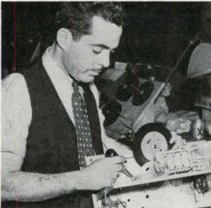
ADJUSTING gang-shaft gears without removing condenser assembly, new method saves time for RCA
