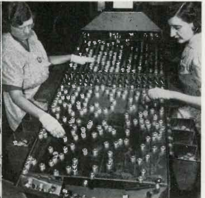
INSPECTION of lamp bases is speeded 400% by Westinghouse sloping "jiggle table." Note "turnover tubes" at middle of table
