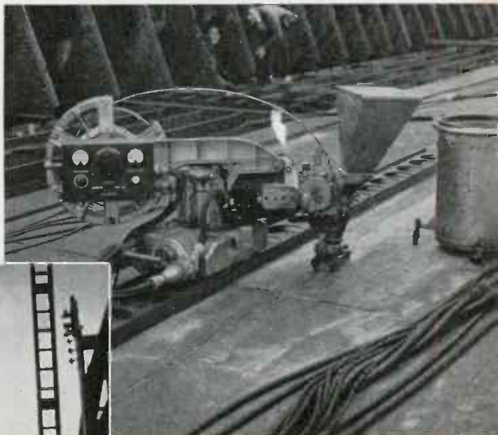
Unionmelt welder, above, automatically welds deck plates of freighter. Diagram shows principle of operation. Thyratrons control arc gap by motor-fed of welding rod. Left: Launching of destroyer U.S.S. Stockton. Below, left: At sea in a rubber boat, plane or ship survivors fly box kite to raise antenna for lifeboat transmitter. Right: Marine radio unit combining twelve separate units in one "packaged" cabinet for Liberty Ship installation. Main and emergency transmitter on left, of 200 watts output on CW, 300 on MCW when used as main transmitter; 50 watts plus as emergency transmitter. Quick-change operation on five predetermined frequencies between 350 and 500 kc is provided. Auto alarm, main receiver and crystal receiver on the operator's right. Federal Telephone & Radio Corp. unit shown.
